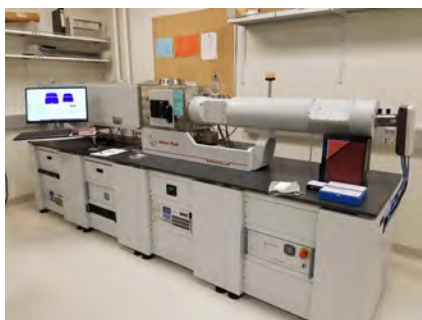
SAXS facility established with NRI funding. The instrument supports a previously underserved user base. The table-top synchrotron alternative broadens access to advanced structural characterization.
