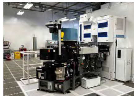
The AMAT Centura cluster tool installed in the AEP core facility on the ASU science park
