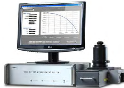
The Ecopia Hall effect measurement system will allow measurements of free carrier concentration, mobility and sheet resistance over a temperature range 80K to 773K.
