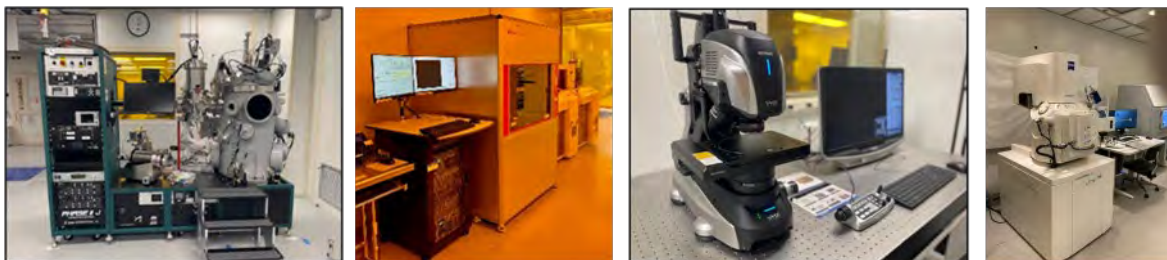
Newly added capabilities at CNF: AJA UHV Multi-Technique Deposition system, Heidelberg MLA150, Keyence Digital Microscope, and 200 mm capable Zeiss GeminiSEM 560
