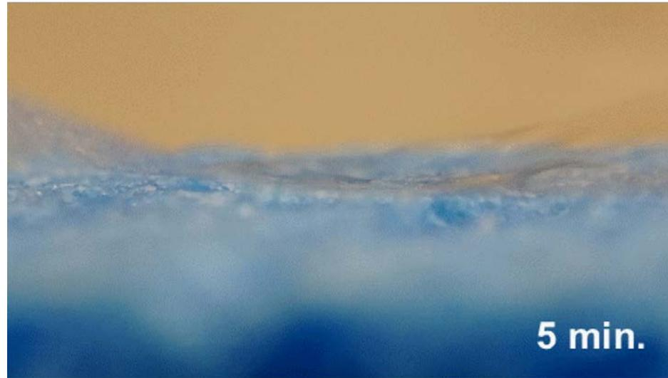
A piece of 0.5 wt.% CNF film exhibits hygroscopicity, swelling and curling with absorbed moisture while resting on a lightly dampened sponge.
