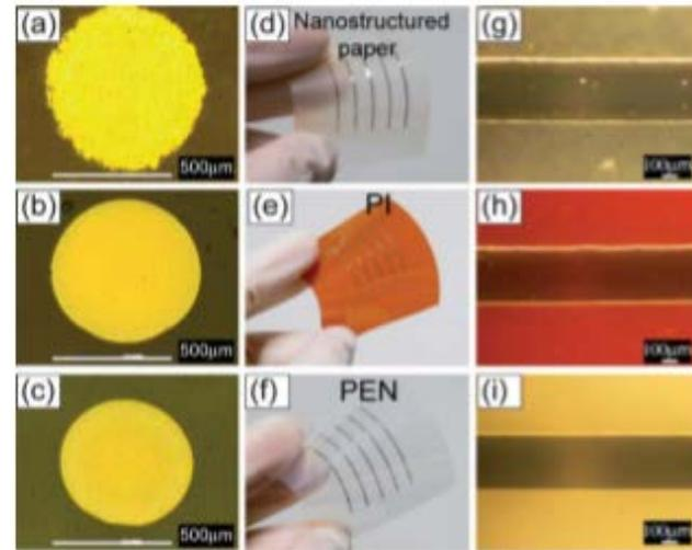
Comparison of inkjet-printed silver nanoparticles on CNF films, polyimide (PI), and poly(ethylene naphthalate). 1<sup>st</sup> column: printed dots; 2<sup>nd</sup> column: printed tracks; 3<sup>rd</sup> column optical images of printed tracks. *Reproduced from Nge, et al., J. Mater. Chem. C 2013*
