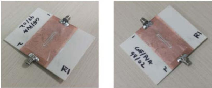
Humidity sensor prototypes consisting of CNF films taped atop coplanar waveguide (CPW) circuits. *Reproduced from Eyebe et al., Sensors and Actuators B: Chemical 2017*
