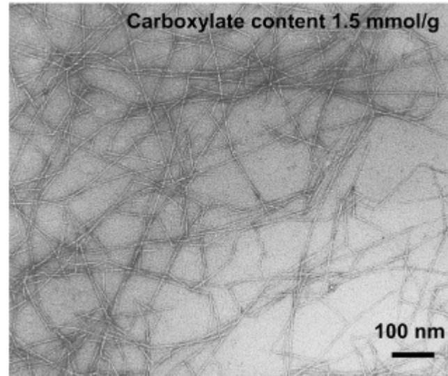
TEM image of aqueous dispersion of 2,6,6-tetramethylpiperidinyloxy (TEMPO)-oxidized CNFs. Reproduced from Saito et al., *Biomacromolecules* 2007.
