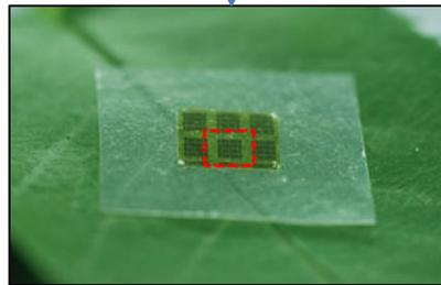
Microwave active GaAs electronic devices on CNF paper. [Yeji Hwan Jung et al. Fig. 3s. CC BY 4.0](#)
