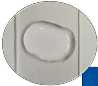
Dish-dried from aqueous 2,6,6-tetramethylpiperidinyloxy (TEMPO)-oxidized CNFs
