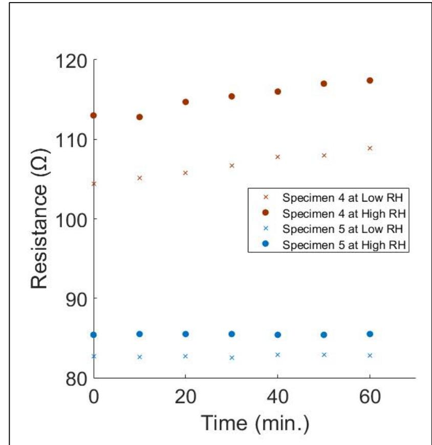
**Specimen 4:** 8% increase in resistance when RH increased from 8-10% to 46%.
