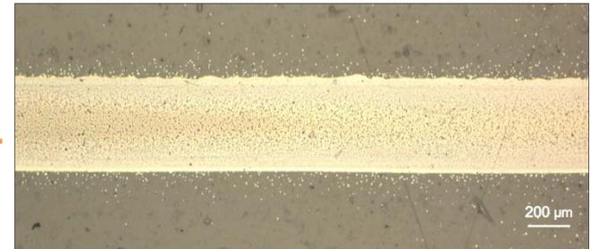
Sintered in oven for 2 hours at 100 °C.
