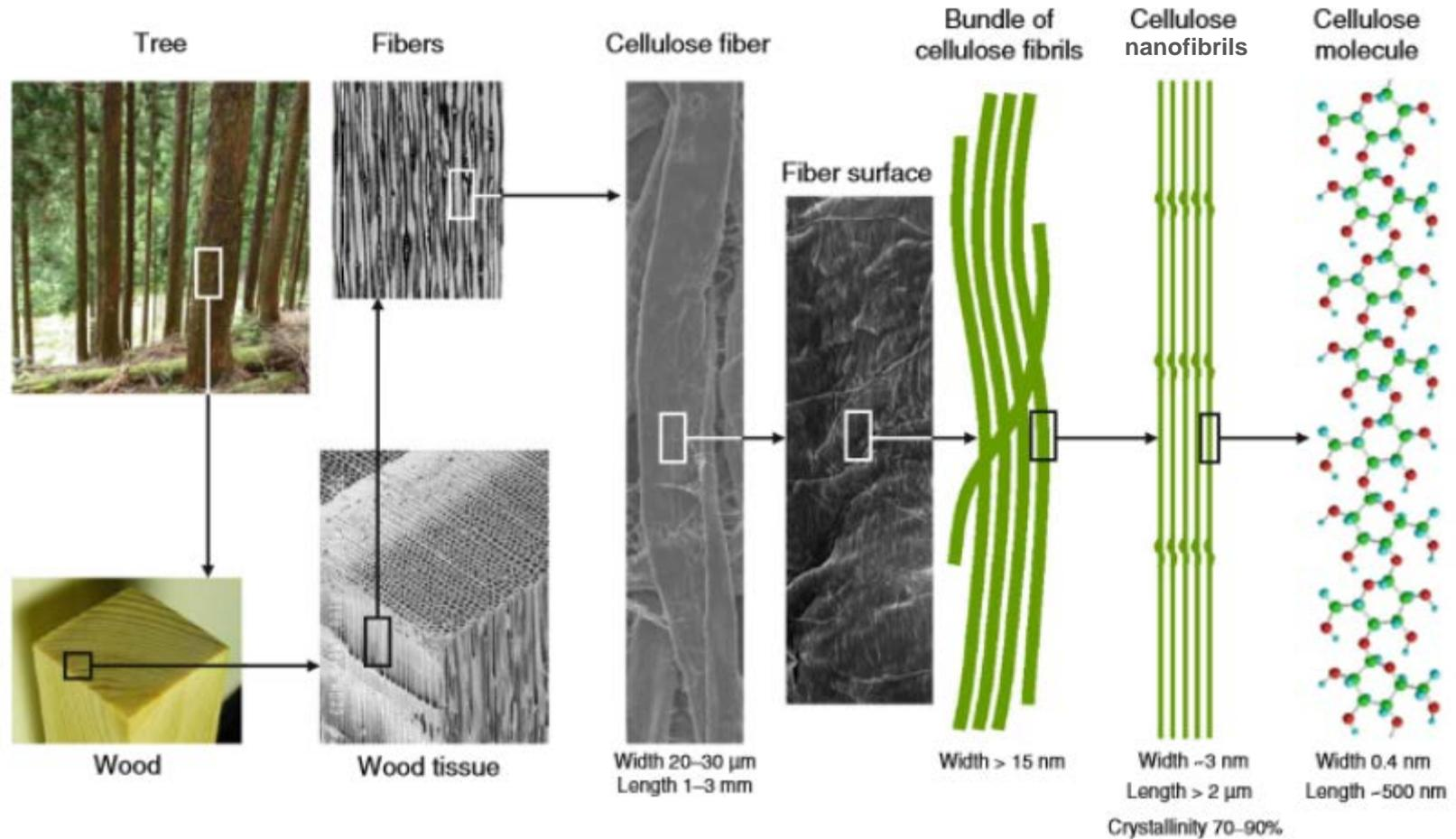
Wood cellulose is composed of bundled cellulose fibrils, which are in turn composed of individual cellulose nanofibrils (CNFs).
