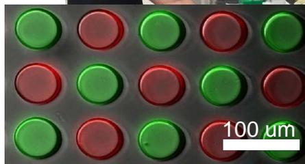
The **Alveole PRIMO/Leica** is targeted at the bio and medical community. It allows to control the chemistry and topography of cell microenvironment and study their impacts on cell development, using a contactless and maskless quantitative photopatterning solution.
