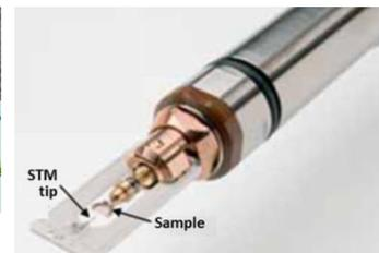
Nanofactory nano-manipulation and electric biasing holder
