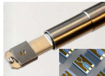
Gas-flow TEM holder can deliver up to 8 pressure-controlled gases (from  $\leq 10^{-7}$  Torr to 1 atm), with local specimen heating
