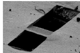
Top and bottom of the cells are removed by FIB milling, leaving a thin slice of the cell volume (80-200 nm)
