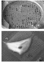
Cells are cultured on EM support grids and vitrified by plunging into liquid ethane
