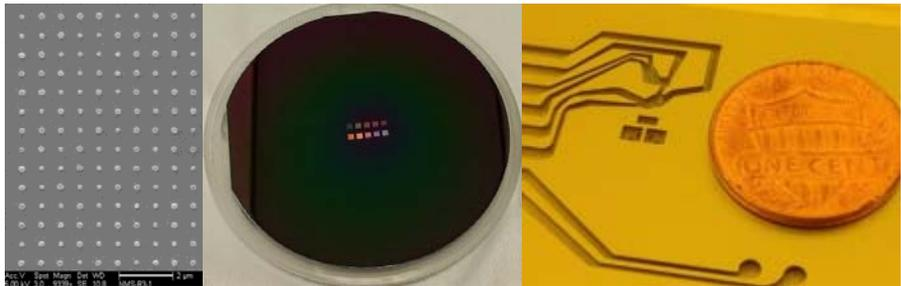
**4" electroformed Ni mold, 200nm features**
