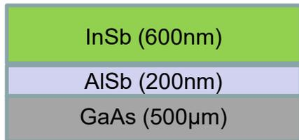
Starting sample (MBE by Bank group) contains lattice mismatch between InSb/AISb and GaAs to introduce defects and decrease carrier lifetime.
