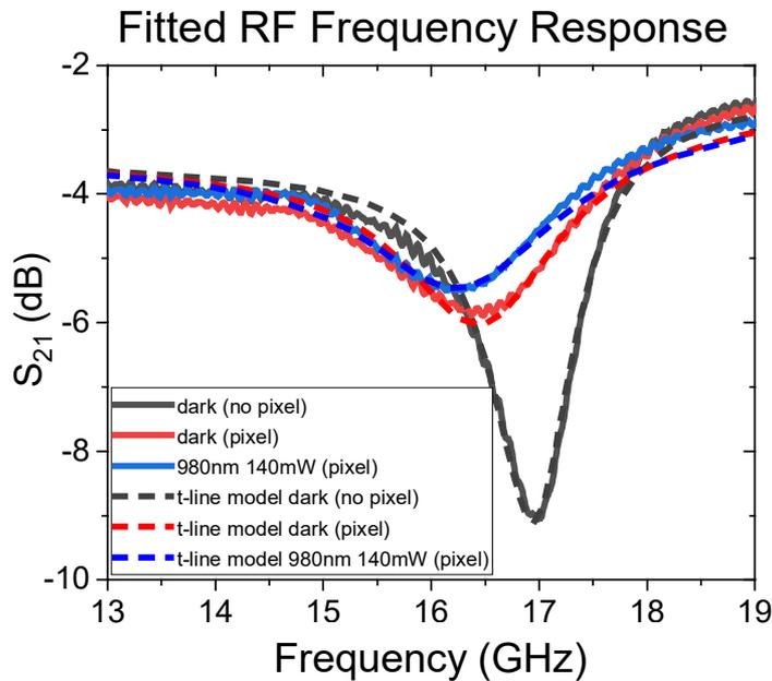
RF transmission fit using model, adjusting pixel conductance and capacitance.
