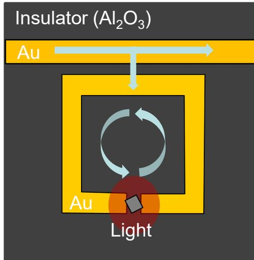
Pixel-loaded SRR responds to light, modulating RF transmission
