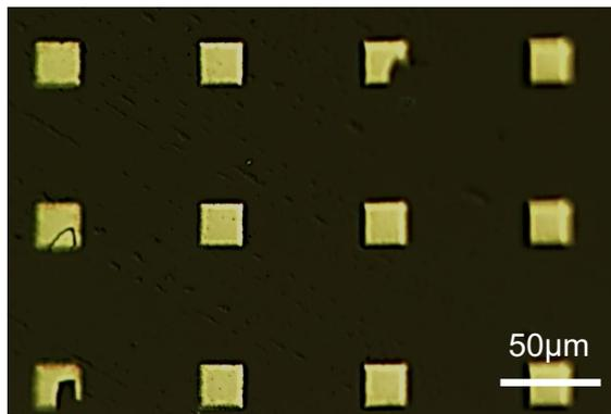
InSb pixel array on PDMS stamp after peel off
