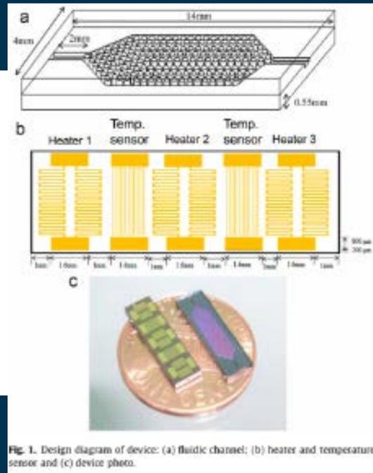
Fig. 1. Design diagram of device: (a) fluidic channel; (b) heater and temperature sensor and (c) device photo.
