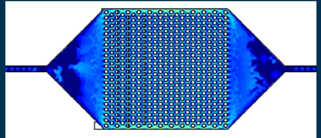
Alternating 50 micron diameter cylindrical posts with sloping inlets and outlets
