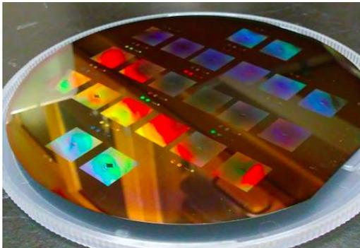
*Large area sub-wavelength diffractive optics, also known as metasurfaces can revolutionize the current state of optical imaging.*
