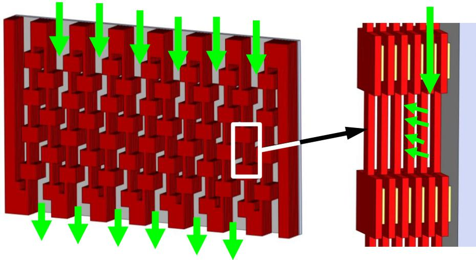
*Layers of structural and sacrificial materials are used to create pores for filtration, separation and chromatography*
