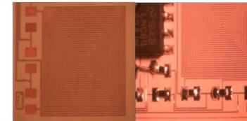
Figure 3. Maskless Lithographic generated Cu/LCP temperature sensor.
