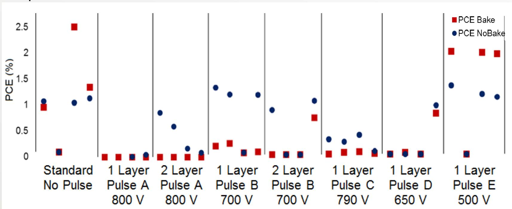
High intensity Pulse (650-800 capacitor voltage) didn't give any improvement efficiency, likely due to thermal damage.
