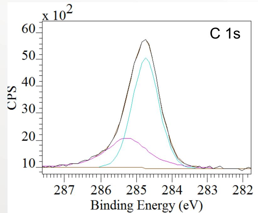
Carbon layer on the pulsed CIS nanocrystal surface,
