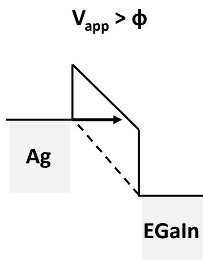
$$J_{FN} \sim V^2 \exp\left(-\frac{4d}{3q\hbar V} \sqrt{2m\Phi_B^3}\right)$$
