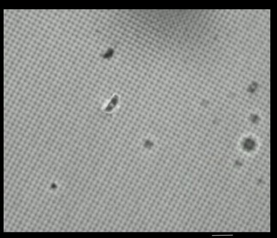
This video illustrates the reaction between the bubble generation and diatom when the algae is added to the surface. The parameters used are laser intensity 100 and scan speed 10000.
