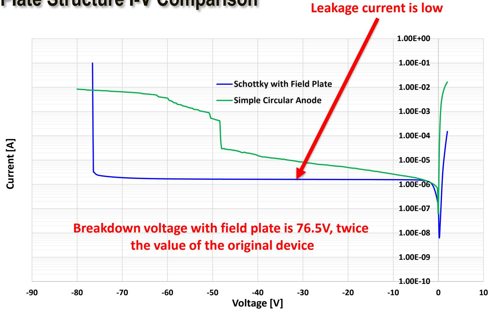
Fig. 16 IV curve final device vs. circular anode
