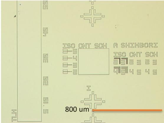
Fig. 9 Isolation alignment marks
