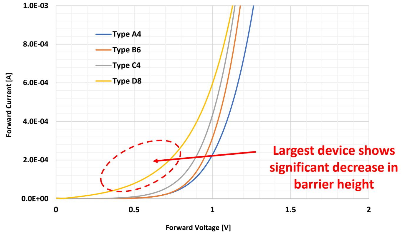
Fig.18 Forward voltage comparison
