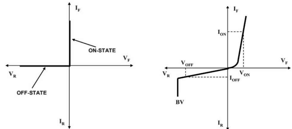
Fig. 1 Power device IV curves
