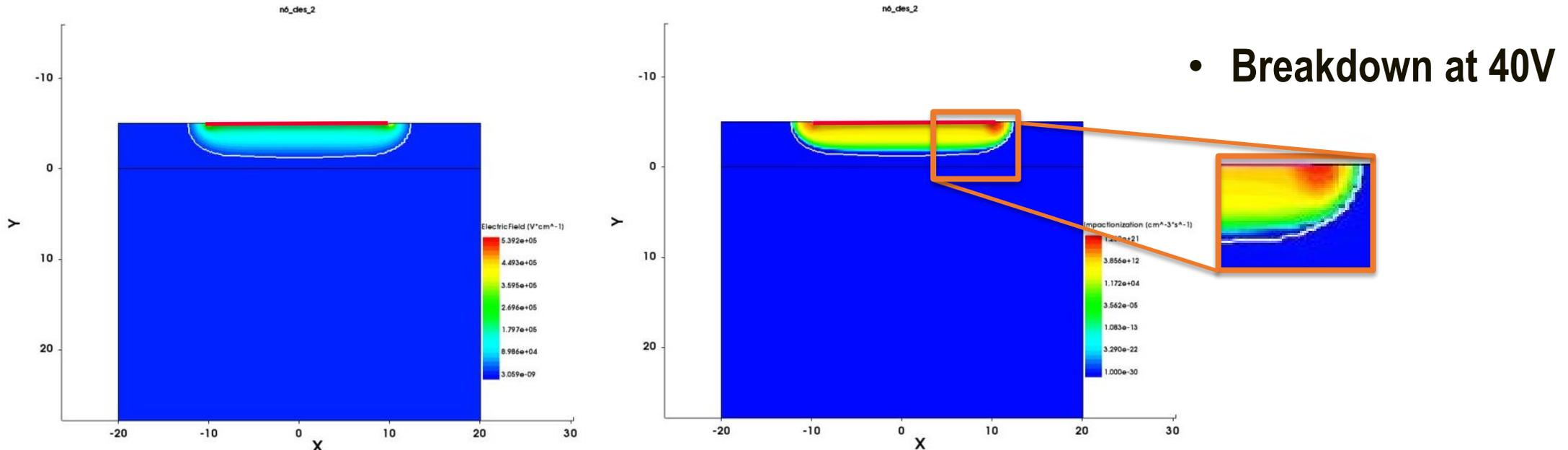
Fig. 4- Circular Diode impact ionization simulation
