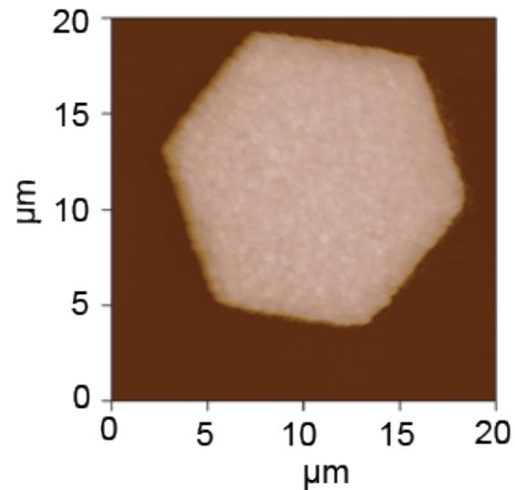
Morphological changes of  $\text{PbI}_2$  crystallites upon reaction with MAI vapor to form  $\text{CH}_3\text{NH}_3\text{PbI}_3$ .
