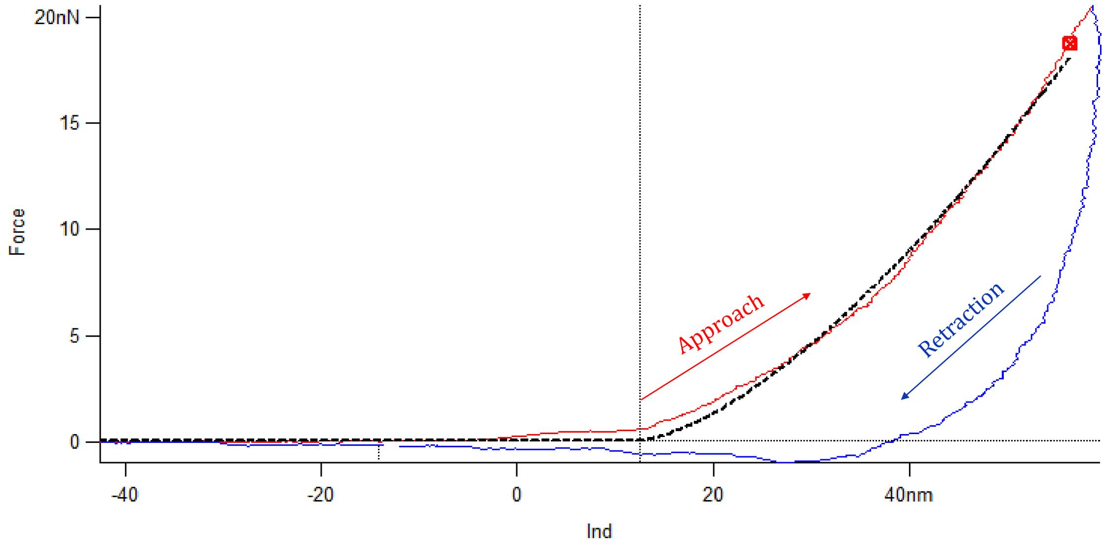
Force-indentation curve for nanogels is shown. Fitting the entire curve with Hertz model (black) gives modulus of 1.70 MPa, but neglects less steep region of curve.
