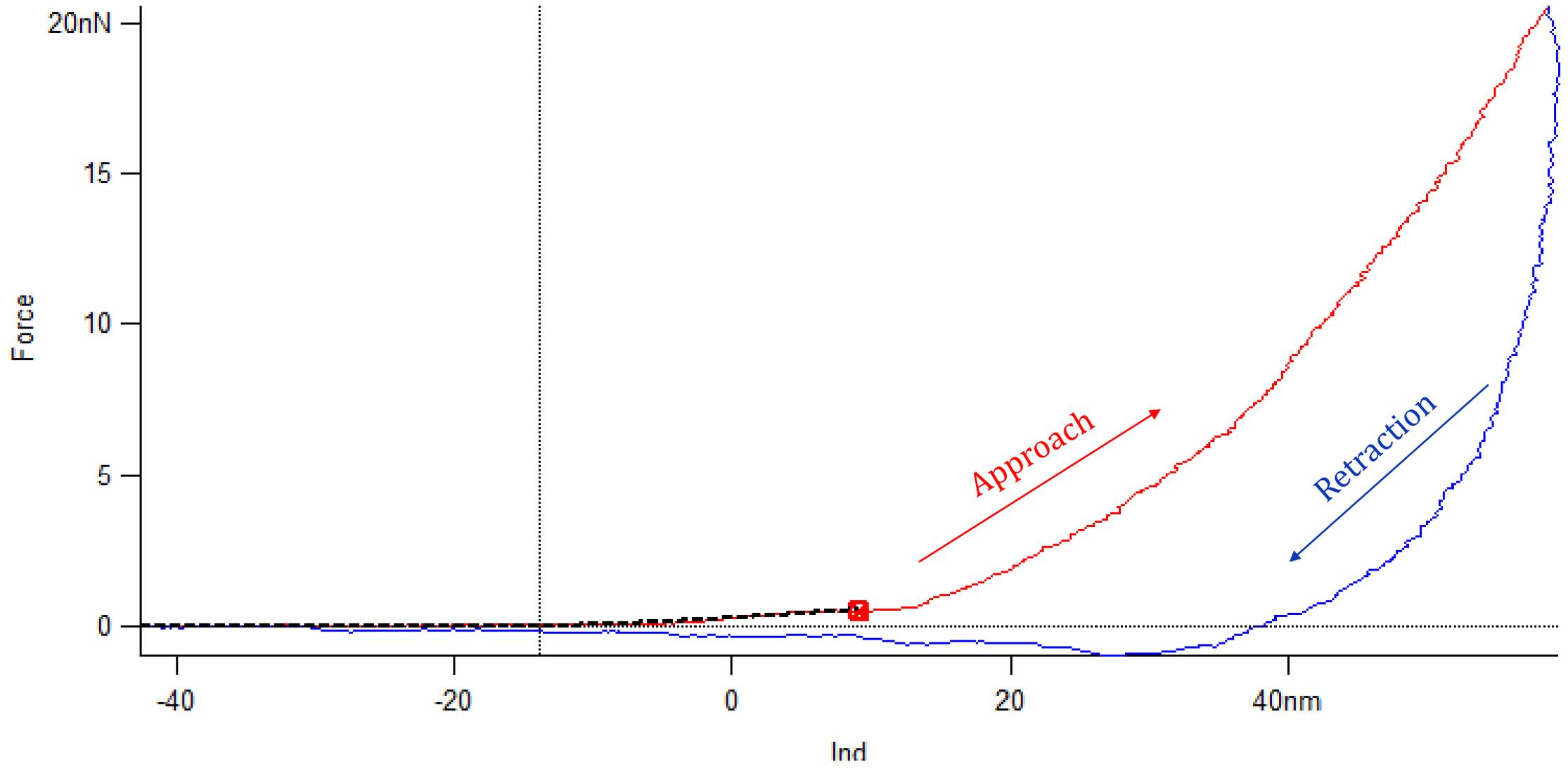
Fitting of 15% of curve captures shallow region to give modulus of 137.31 KPa, suggesting a two-component system
