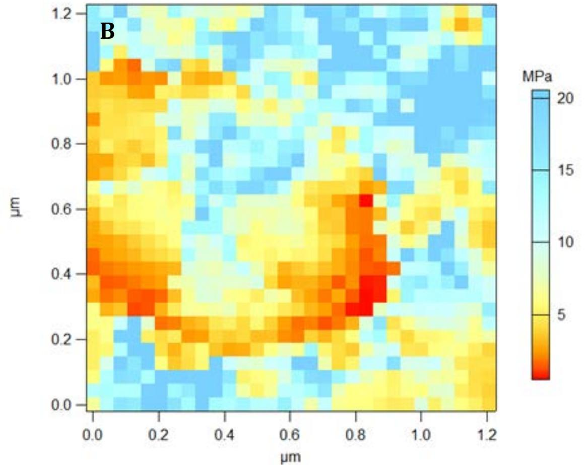
Support for a two-component system is seen in elastic modulus map (B) of aggregate nanogels (A). Aggregate measures approximately 1  $\mu\text{m}$  in diameter and 150 nm in height. Lower modulus influenced by dextran (KPa)<sup>7,8</sup>, while higher by lysozyme core (0.5 GPa)<sup>9</sup>.
