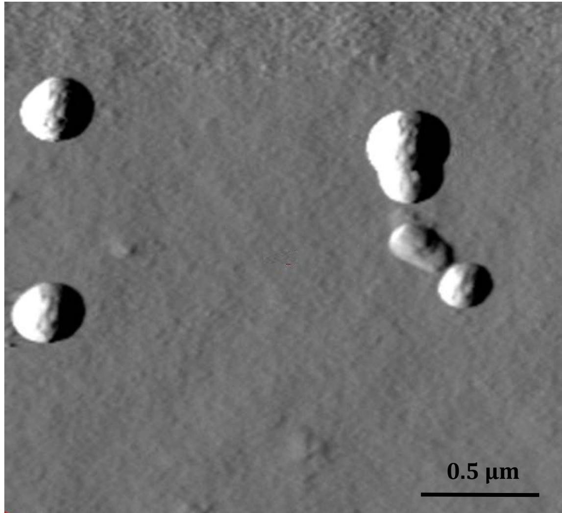
AFM topographical images of smaller nanogels taken with cantilever with silica probe reveal nanogels successfully grafted to APTES treated surfaces. Average nanogels measure approximately 200 nm in diameter and 30 nm in height.
