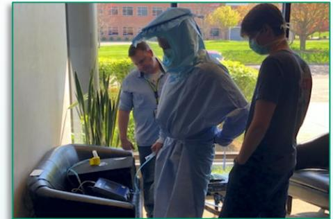
Integrated powered air-purifying respirators (PAPRs) retrofit kit
