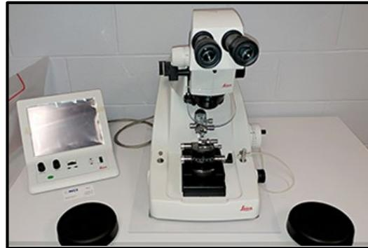
Leica UC7 Ultramicrotome
