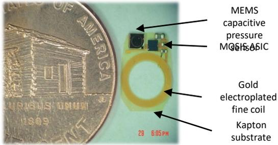
**Wireless IoT Strain Sensor System for Spinal Fusion Monitoring**
