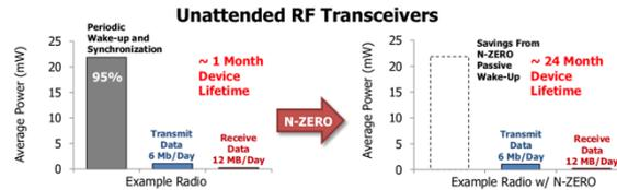
**Figure 2.** Reference transceiver lifetime without (left) and with an N-ZERO wake-up (right) for an existing mesh network radio when network traffic is sparse [1]. N-ZERO systems do not drain the battery for scheduled wake-up and synchronization.
