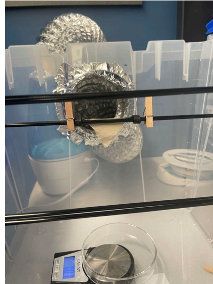
Completed fog collection setup, before fog is turned on
