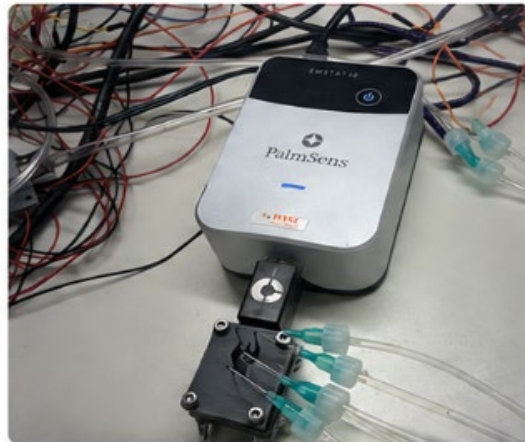
Microfluidic Biofilm Chamber with Integrated SPE Working Electrode
