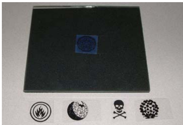
(1) Put photoresist film under the pattern and glass.
