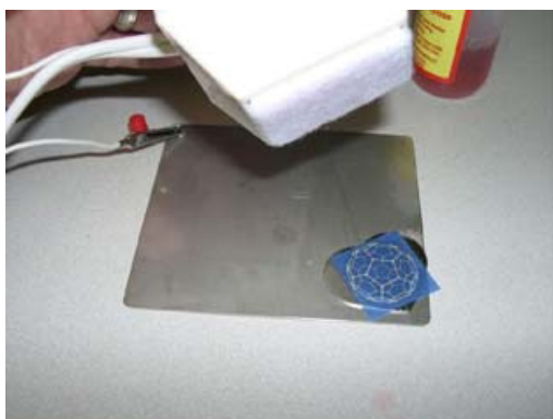
(7) Put electrolyte on photoresist and felt pad; put etcher over dog tag for 10 seconds.
