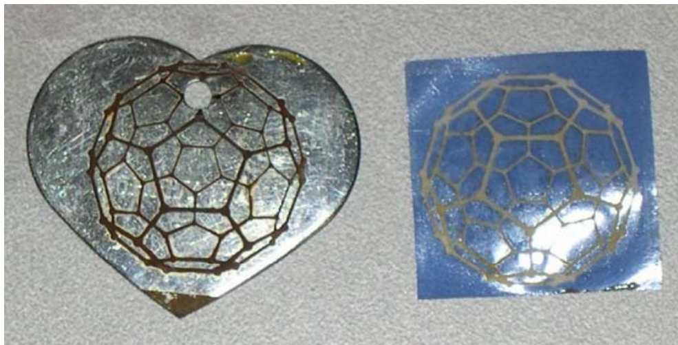
(9) Etched dog tag with oxide pattern and photoresist film.
