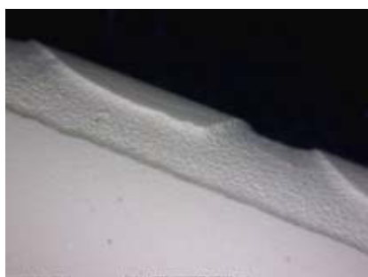
This picture shows the dot structures with the mask removed. The sidewalls are very sloped.
