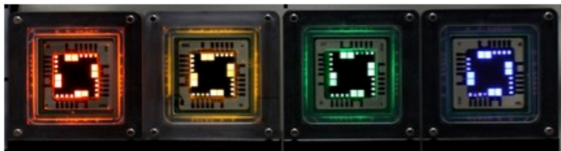
Figure 3: Quantum Dot based Light Emitting Diodes (QLEDs) are currently being developed for displays and lighting applications. In the photo above, we are seeing QLEDs manufactured by QDVision.
