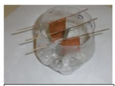
Figure 1: Electro deposition Cell
