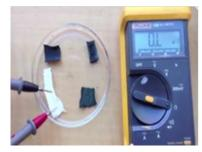
**<u>Step 7a</u>**: Measure the conductivity of the 4 cotton fabric samples. Begin with the untreated cotton fiber fabric square sample as the control. Record the resistance in your data table.
