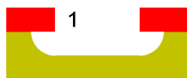
Figure 1: An isotropic etch is a shape which undercuts the substrate below the mask at the same rate as it penetrates into the substrate making a wider channel than may be expected.
