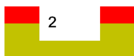
Figure 2: An anisotropic etch forms a square shaped hole. Some single-crystal materials, such as silicon, exhibit anisotropic etching in certain chemicals. Anisotropic etching —in contrast to isotropic etching—means different etch rates in different directions in the material. (Image from Wikipedia)
