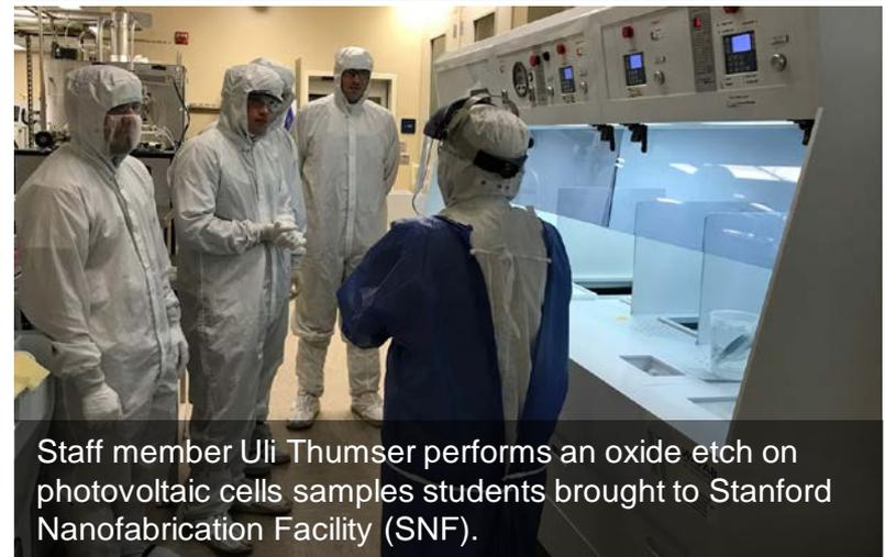
Staff member Uli Thumser performs an oxide etch on photovoltaic cells samples students brought to Stanford Nanofabrication Facility (SNF).
