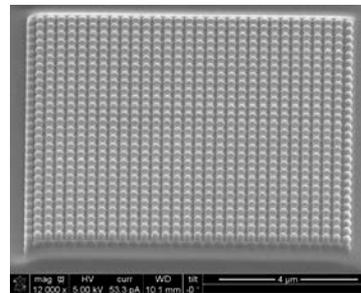
Final stamping die, 10 x 10 μm with 320 nm pitch
