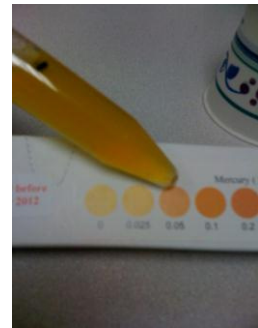
Positive test for mercury in water.
