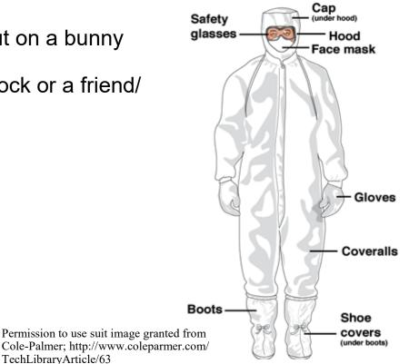
Cleanrooms are facilities where the air is filtered on a continuous basis to remove particles like dust, pollen, microbes, etc. These facilities are commonly used to manufacture electronic devices—like chips— and to do research. Why are cleanrooms needed? Even the tiniest particle can affect the making of a chip or a device. The NASA Hubble Space Telescope did not perform as designed because of a particle smaller than 0.5 microns. The diameter of a bacterium is 0.2 to 2.0 microns.
