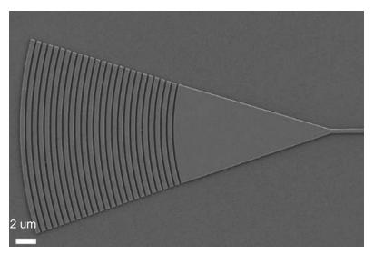
The couplers guide light through this waveguide. The HUDS pattern controls light propagation within the structure.
