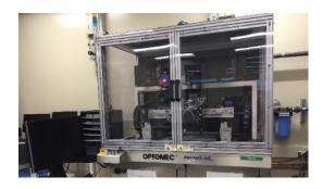
The Optomec Aerosol Jet AJ 300 is a non-contact, direct-write system with the ability to conformally print just about any ink, to feature sizes as small as 10 um.
