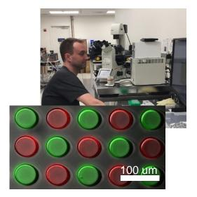
The Alveole PRIMO/Leica is targeted at the bio and medical community. It allows to control the chemistry and topography of cell microenvironment and study their impacts on cell development, using a contactless and maskless quantitative photopatterning solution.
