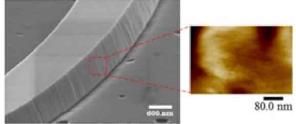
(a) Zoomed-in angled-view SEM image of the microring resonator. (b) 2D AFM scan of sidewall.
