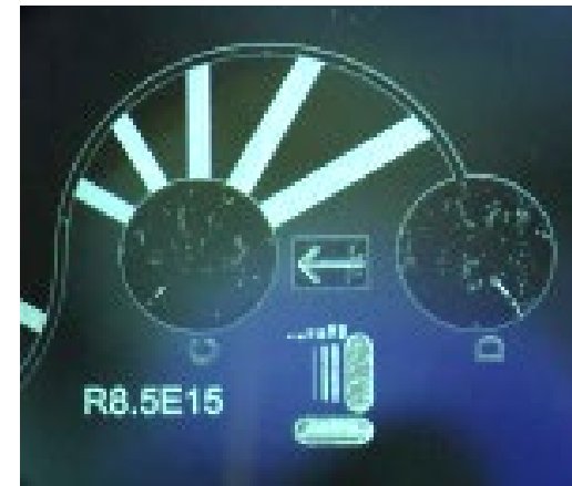
Figure 2: Phase contrast microscope image shows the microfabricated channels after casting into PDMS. Shallow channels reflect upright light more than deeper channels.
