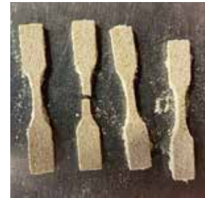
Green parts from SLS machine.
