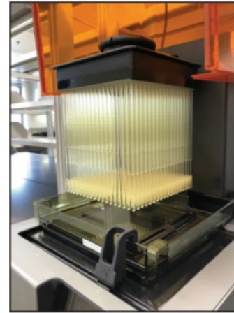
Top Left: Completed print of 324 adult swabs using Formlabs Form2 with Surgical Guide resin. Top Right: PurFlock (Puritan Medical Products, LLC) test swab (a) compared to 3D-printed pediatric (b) and adult (c) swabs.
