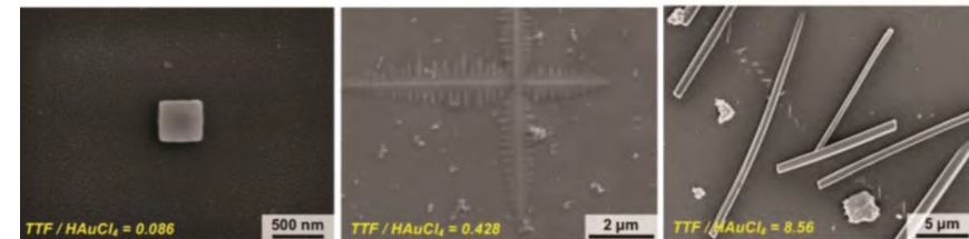
SEM images of nanohybrids synthesized by mixing tetrathiafulvalene (TTF) and HAuCl 4 solutions at different flow rate ratios
