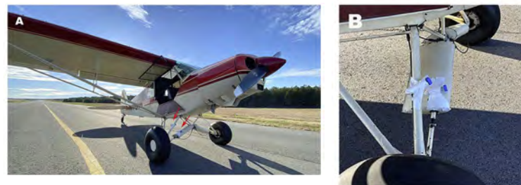
Exhaust samples were trapped on EM supports after exiting the aircraft exhaust pipe
