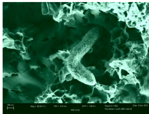
SRB Desulfovibrio vulgaris in biofilm formed on the surface of a carbon steel sample
