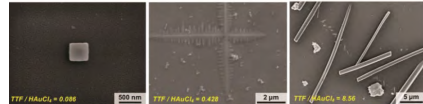
SEM images of nanohybrids synthesized by mixing tetrathiafulvalene (TTF) and \text{HAuCl}_4 solutions at different flow rate ratios
