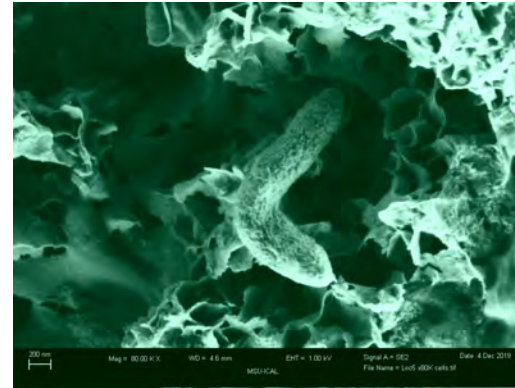
SRB Desulfovibrio vulgaris in biofilm formed on the surface of a carbon steel sample
