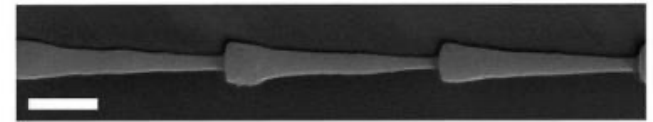
SEM image of a nanowire with three geometric diodes in series (Scale bar = 200 nm)
