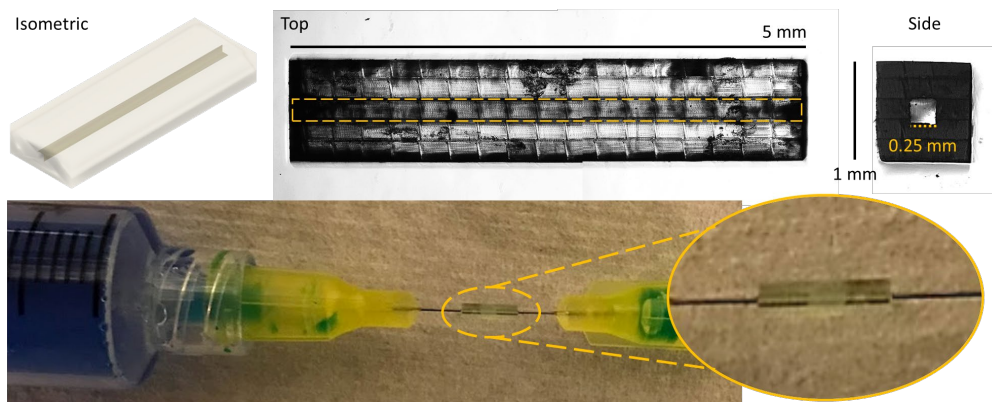
An isometric view and brightfield images (top and side views, 4x) of the 3D printed construct are shown highlighting the channel in yellow. The physical construct was perfused via 32 gauge needles with no leakage when sealed.
