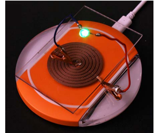
Cu-Ag NW filament was printed into an inductive charging coil. The coil powered an LED when paired with a wireless charging dock.
