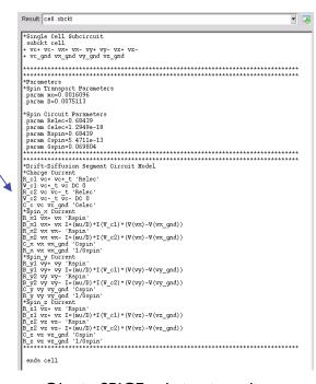
Obtain SPICE subcircuit netlist describing spin & electron transport in channel
