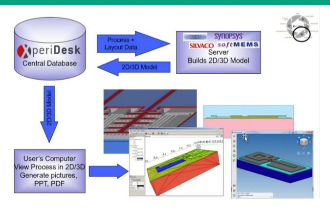
A knowledge capture repository for process flows which can generate 3D renderings of devices to be fabricated.
