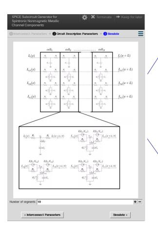
Use developed compact circuit model for spintronic transport
