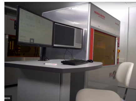
The Heidelberg direct write lithography system allows great flexibility to pattern a wide range of substrate materials.
