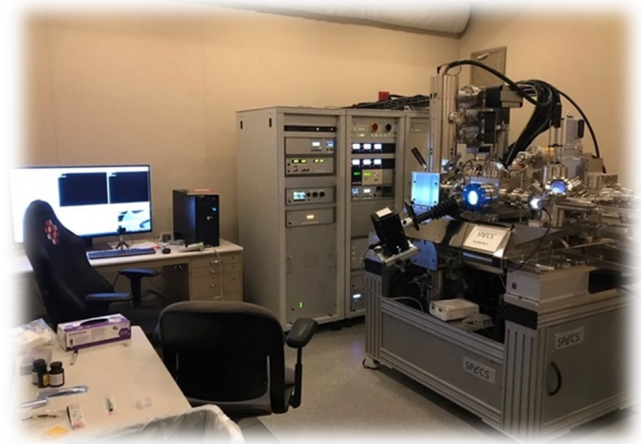
New MRI-funded LEEM System
