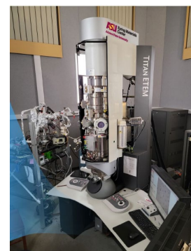
The Titan environmental TEM can record high speed video at liquid nitrogen temperatures.
