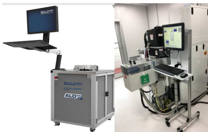
The Lesker ALD150LE (left) and the SPTS Rapier (right) were purchased during the fifth year. Both have been installed. The ALD system is available to users while the deep silicon etch system is in acceptance testing.
