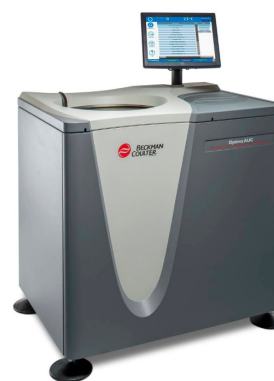
The AUC system is capable of 1000g acceleration and operates up to 60,000 rpm.
