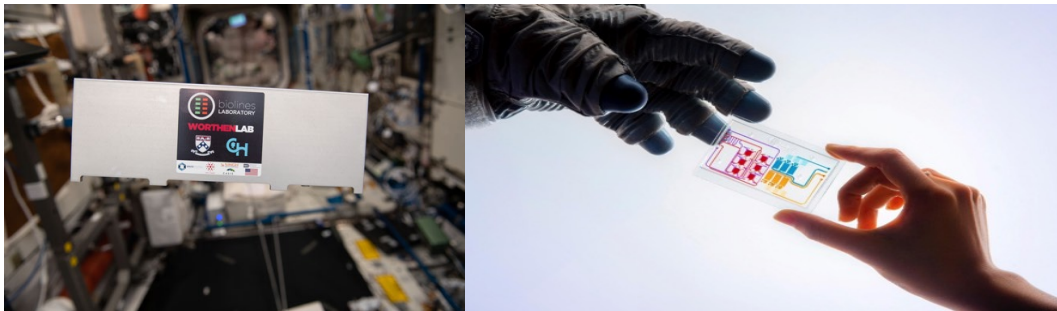
MANTH fabricated microfluidic device for lung infection studies floating in the ISS.
