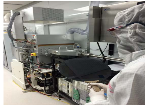
Figure 1: Canon Nanotechnologies Dry Etch Development scaling up for use on 300mm wafers
