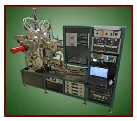
54 National Nanotechnology Coordinated Infrastructure Capability to deposit ultra-high purity superconductors, normal metals, dielectrics
