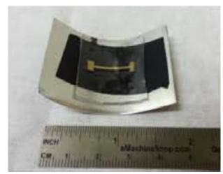
A bent microcracked gold conductor under moderate compression
