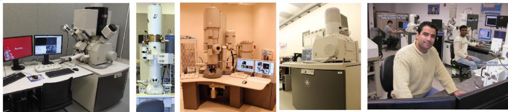
Electron microscopy: FEI Helios 660 SEM/FIB, JEOL and FEI TEMs, FEI and Zeiss Environmental FE-SEMs, other FE-SEMs
