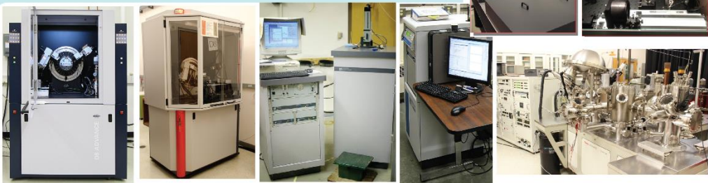
Materials characterization: x-ray diffractometers, spectroscopic ellipsometers, squid magnetometer (QD MPMS), physical properties measurement system (QD PPMS), XPS and Auger surface analysis, ultrafast optical spectroscopy
