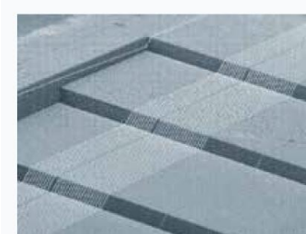
Silver lines printed over a 3D substrate.
