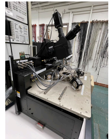
DC probe station
